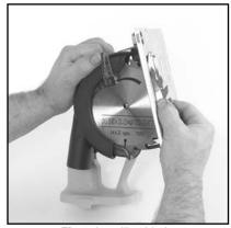
Fig 6. Installing blade.
